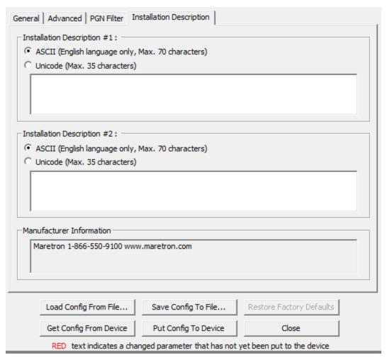
Figure 7 - NBE100 Installation Description Tab
