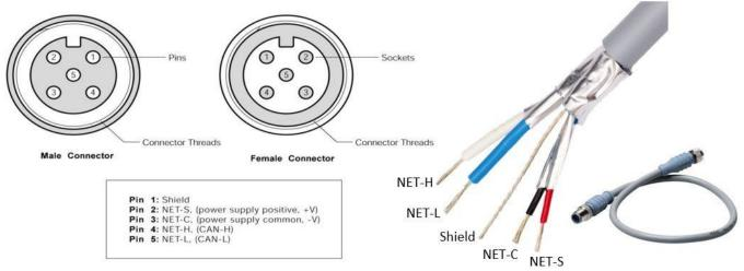
Figure 2 – NMEA 2000<sup>®</sup> Connector Face Views
