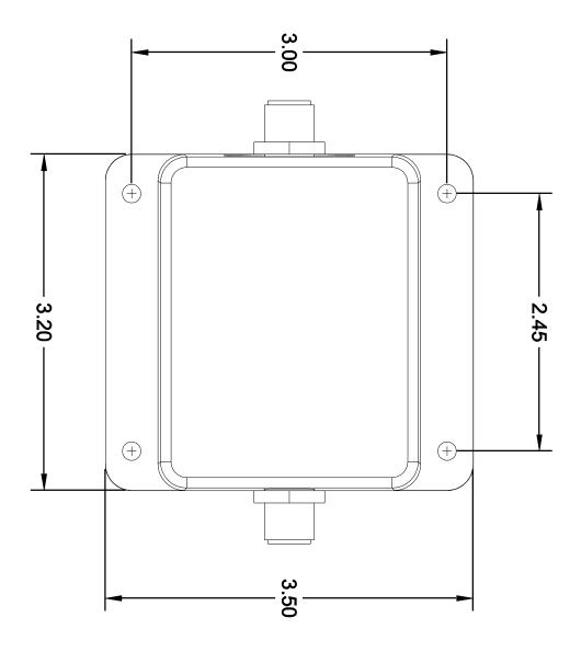
Figure 8 – Mounting Surface Template
