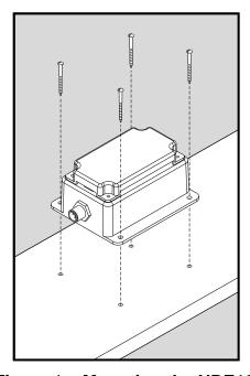
Figure 1 - Mounting the NBE100
