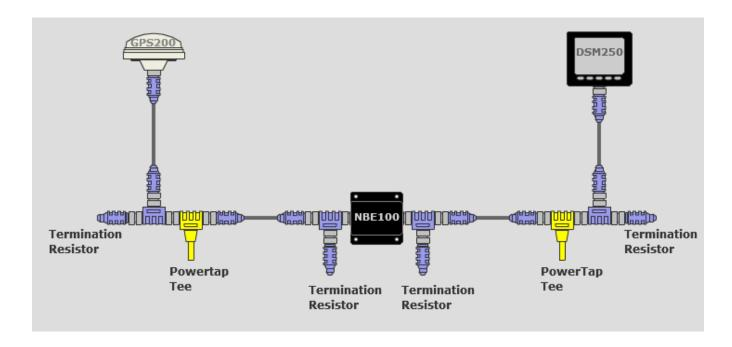
Figure 3 – NBE100 Connection Diagram
