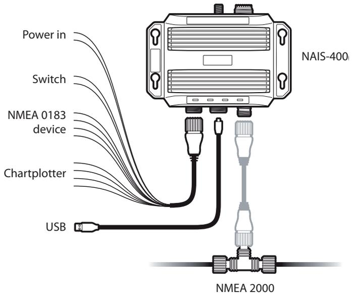
Figure 3 Electrical connections to the AIS transceiver
