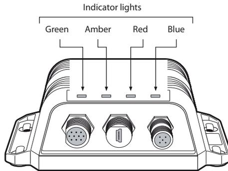
Figure 13 Indicator location on the AIS transceiver unit
