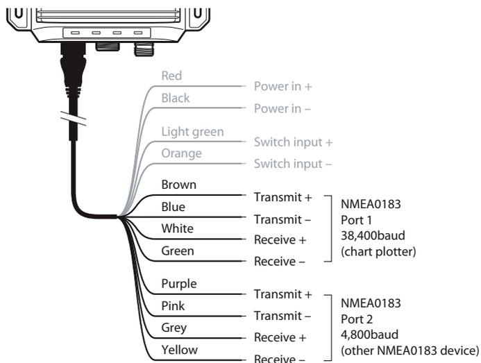
Figure 11 Connecting to the NMEA 0183 data port
