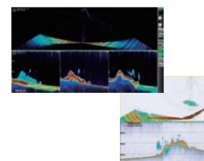
WASSP gives you wide-angle 120° port-starboard view of the seafloor and water column with 112 beams per ping. The viewing span is over 3 times sea depth, and WASSP can profile an area over 100 times faster than a single beam system.
