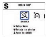
After performing the software upgrade, a SABIKI icon will appear in the turn menu. The SABIKI mode is only user selectable if the current speed is below 5 knots. Once SABIKI mode is selected, the course can be set with the Roto knob and the arrow keys.
