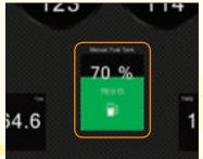
Manual Fuel Tank display in Instrument mode
