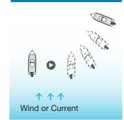
In order to keep the same direction it is not sufficient to just reverse the engine and move astern. The steering has to be constantly adjusted to keep direction.
