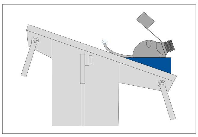
The unit's cable can be routed protruding from the rear of the base or underneath the base as shown below:
